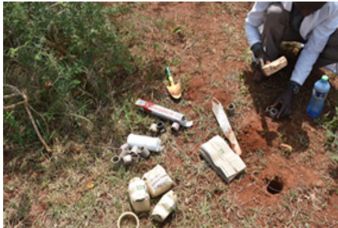
Plate 13: Bulk Density Soil Sampling
