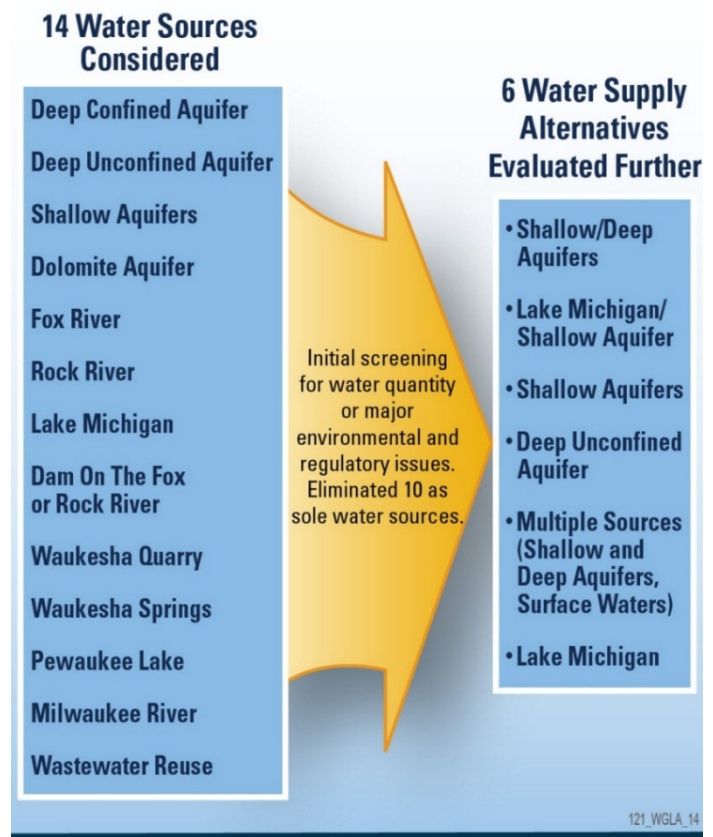
EXHIBIT 11-3 Water Supply Alternative Screening
