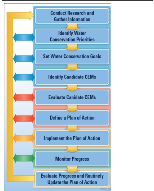
FIGURE ES-1 Water Conservation Planning Process
