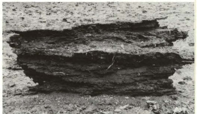
FIG. 59. Stranded portions of 1 m diameter yellow cedar log partially destroyed by both Bankia and Limnoria activity, mainly the latter.
