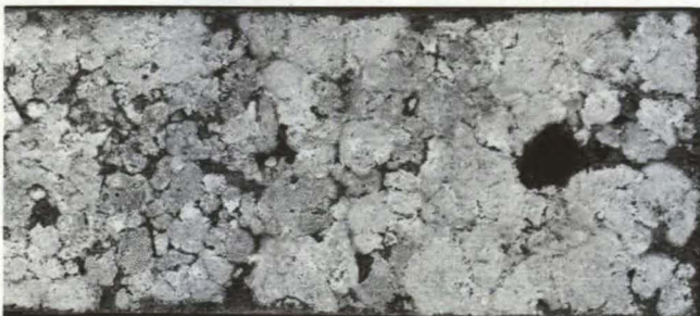
FIG. 54. The bryozoan, Schizoporella unicornis , completely covering a 15 × 6 cm test panel, preventing borer attack.
