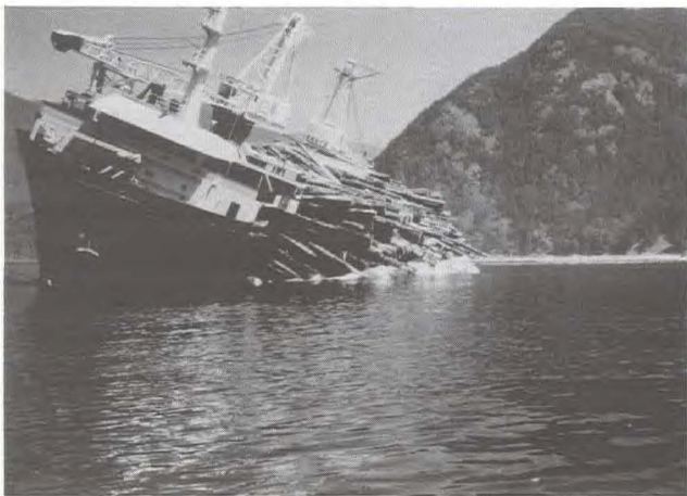
FIG. 43. Typical British Columbia log barge discharging its load. (Council of Forest Industries photograph)
