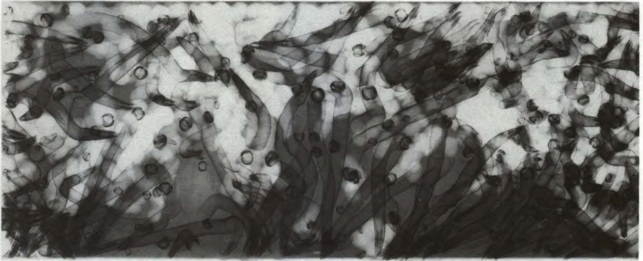
FIG. 26. X-ray photograph of a fir panel (2 × 10 × 20 cm) attacked by Bankia setacea in Ladysmith Harbour from August to December, 1952. (Photograph by H. Duncan. From Quayle 1956)
