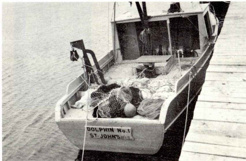
The M/V "Dolphin No. 1", fully rigged with trawl aboard ready for pair midwater trawling
