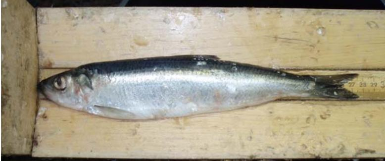
1. Herring are measured on a non-offset measuring board, with the snout abutting gently the headboard.
