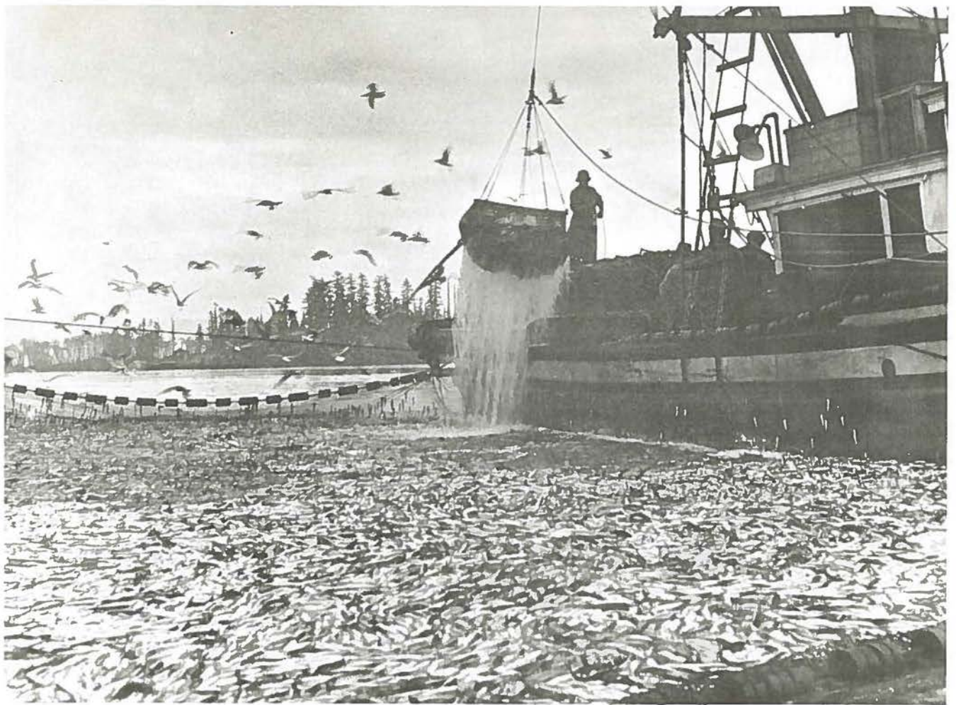
A power winch operates the brailer or huge scoop used to take the thousands of herring from the net. Gulls hover and swoop down on the catch.
