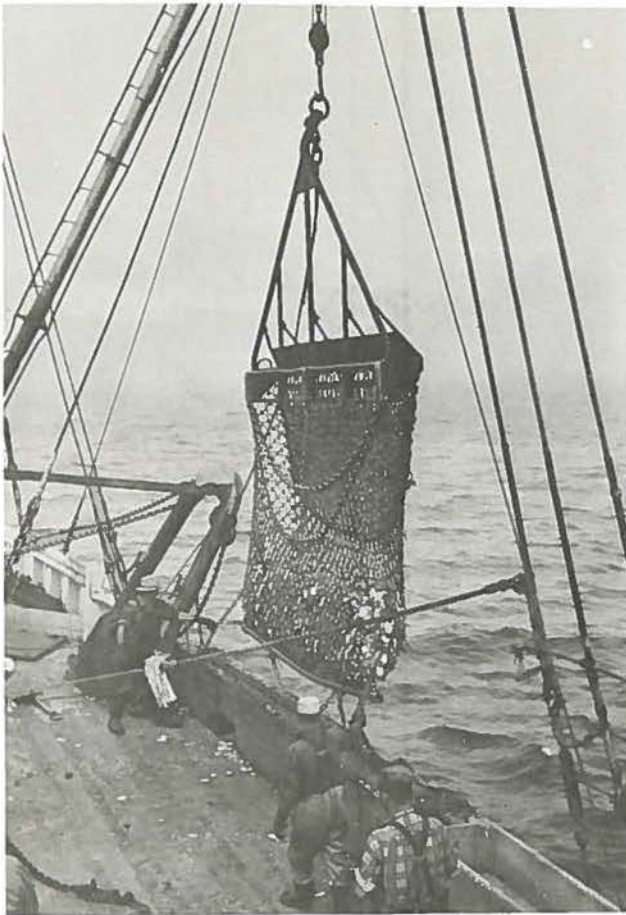
Fig. 5. - Bringing aboard a 12-foot offshore scallop drag after a 20-minute tow on Georges Bank. Empty drag weighs 1400 pounds, with a full catch as much as 8,000 pounds.
