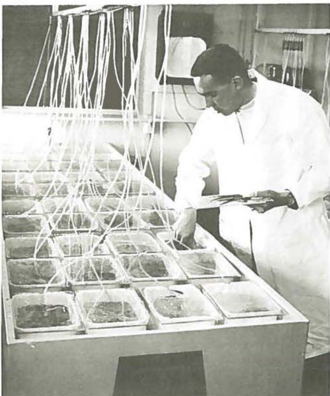
Laboratory assistant checks the condition of ammocoetes and trout subjected in bioassay test to varying concentrations of lampricide.
