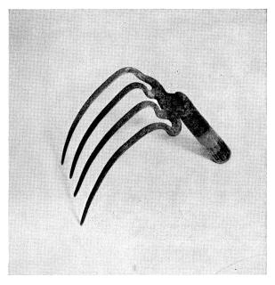
FIGURE 2. Bloodworm fork. The types are 9 to  $10\frac{1}{2}$  inches long, tapering from  $\frac{3}{4}$  inch at the base to  $\frac{1}{2}$  inch near the tip. Most diggers have them made from ordinary garden forks. (Photo by P. W. G. McMullon).
