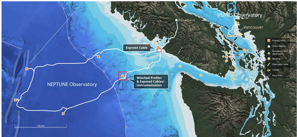
Figure 1. Ocean Networks Canada NEPTUNE Observatory areas of high risk to trawling. Additional caution should be exercised in areas indicated with a red box. (Bathymetry Data Sources: Saanich Inlet and Strait of Georgia bathymetry from Canadian Hydrographic Service; USGS Cascadia DEM report 99-369; University of Washington (UW), School of Oceanography, R/V Thomas G. Thompson , Multibeam cruise data - funding provided by KECK Foundation and UW; Plate Boundaries: Adapted from Dragert et al. Science, May 2001. Map adapted from original by: Center for Environmental Visualization, UW School of Oceanography.)
