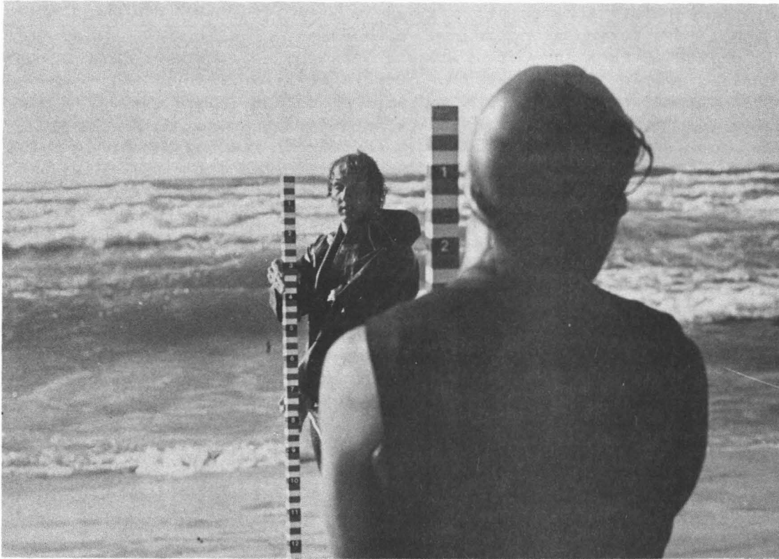
Photo 5.1 Beach profiles were surveyed using the pole-and-horizon method. The change in elevation between two vertical staffs is measured by levelling on the horizon. This is a modification of the method described by Emery (1961). The elevation difference between the staffs in this photograph is -9 cm.
