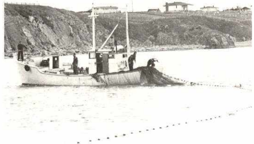
FIG. 27. Trapnet longliner adapted for ringnetting. This technique has proved effective for harvesting capelin and is now being used in Newfoundland waters.
