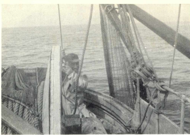
Tow rope is secured to drum and fisherman brings up cod end by hand.
