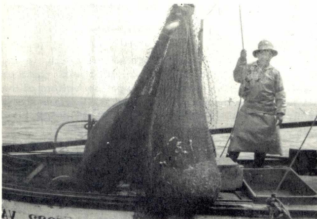
Cod end is drawn from the water after having been thoroughly rinsed .
