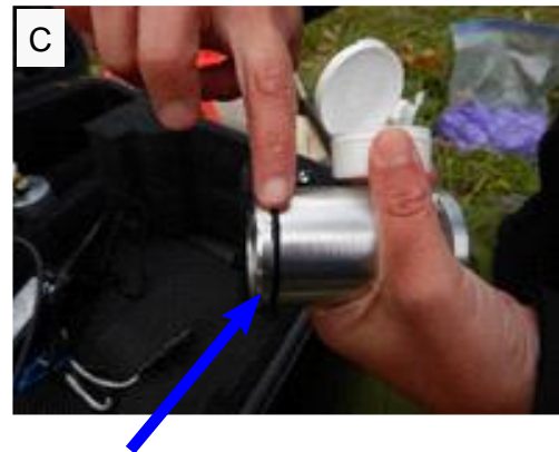
Rubber O-ring on the Inlet Stage
