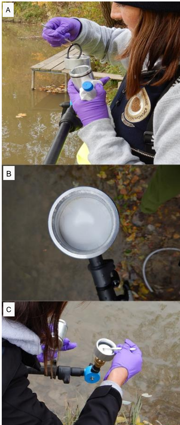
Figure 2.3. Filter placement in the housing. Remove of the flat rubber ring that is on top of the metal mesh (A), put the filter in the final stage on top of the mesh (B) then place the flat rubber ring on top of the filter (C).
