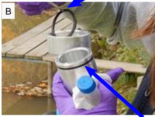
Rubber O-ring on the Inlet Stage
