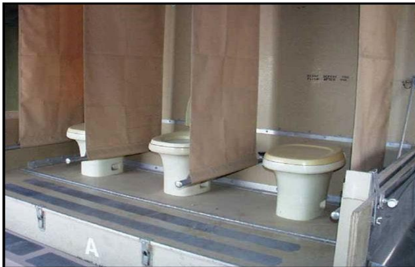
Figure 10.15. Field Deployable Latrine
