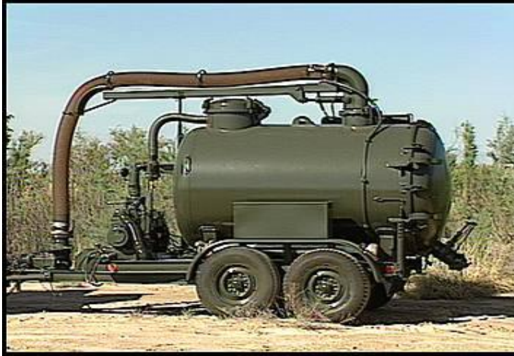
Figure 9.2. Wastewater Disposal Trailer
