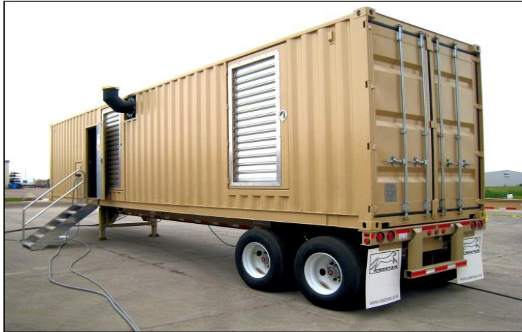
Figure 7.8. Interim Power Unit (IPU)
