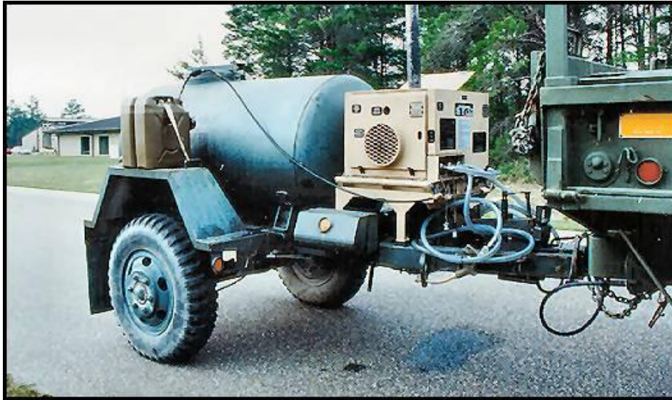
Figure 8.7. 400-Gallon “Water Buffalo” Trailer With Chiller Attached
