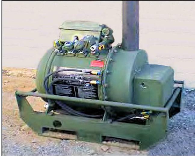
Figure 11.9. WH-400 Water Heater
