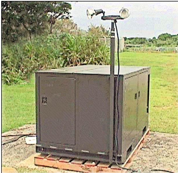
Figure 7.10. Remote Area Lighting System (RALS)
