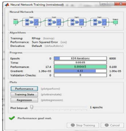
Figure 9. Performance characteristics of the neural network in the training backpropagation
