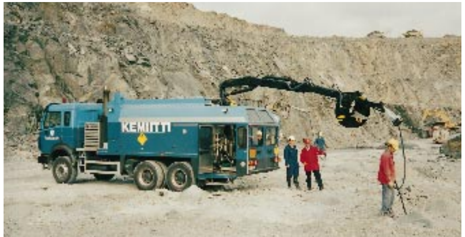
Vihtavuori's efficient and environmentally sound Kemiitti 510 emulsion explosive was put into use at the Outokumpu Chrome mine in Kemi, Finland.
