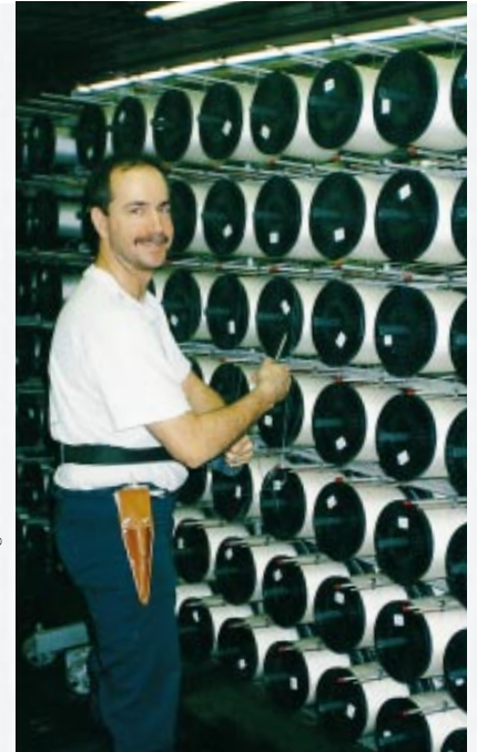
Robert Daly, warper operator, loading new warp yarn on creel in Canton.
