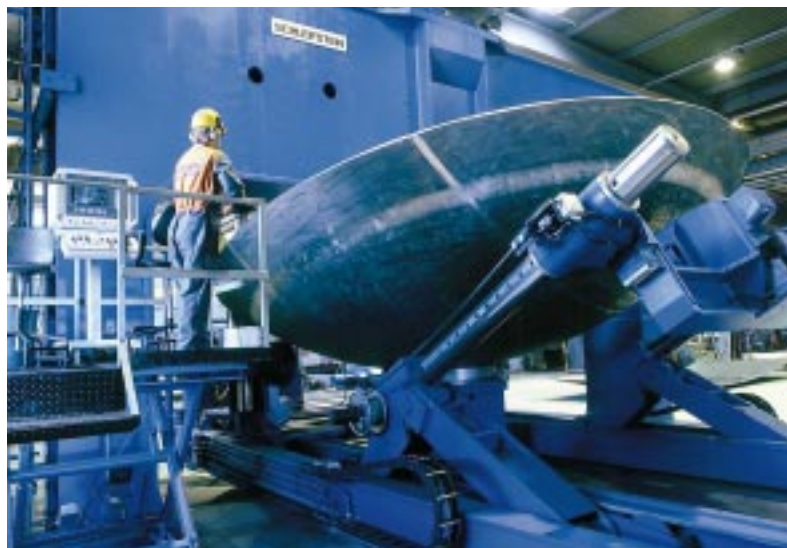
The new hydraulic press at the Halikko Works is capable of manufacturing tank dished ends up to 10 metres in diameter.
