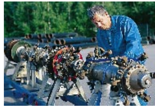
Underground natural gas pipelines are cleaned and inspected by using pieces of equipment known as "pigs" that move through the pipeline with the flow of natural gas.
