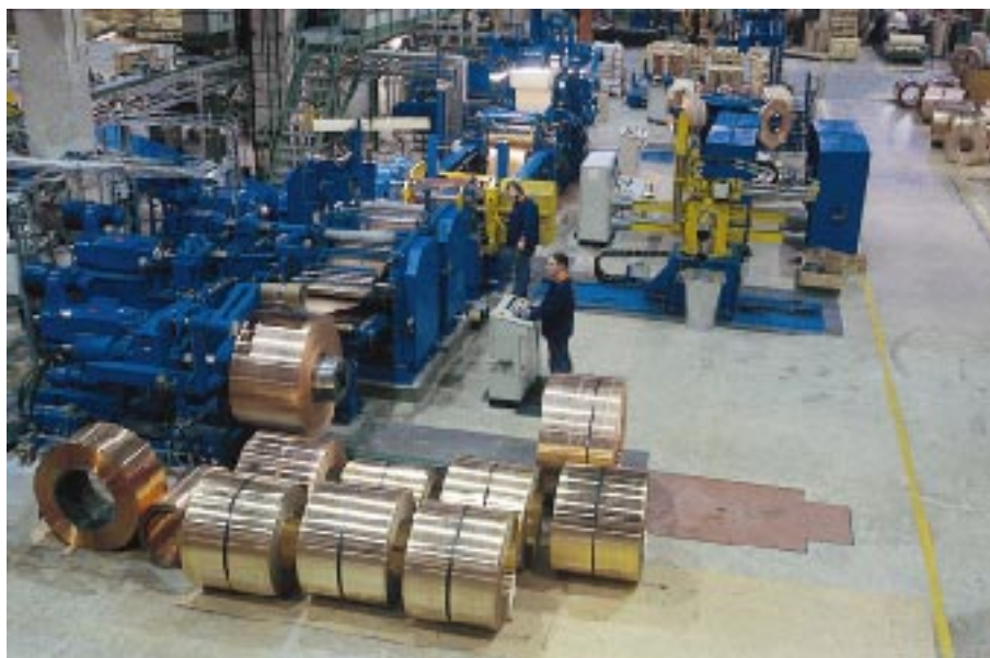
The Pori rolling mill is making preparations for production of the Nordic Gold alloy for the euro coins to be introduced in 2002 and the blanking mill for the fabrication of the coin blanks.
