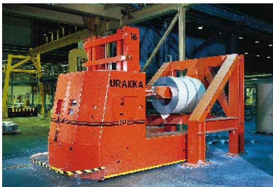
Coils are transferred at the cold rolling mill by 16 automatic guided vehicles.
