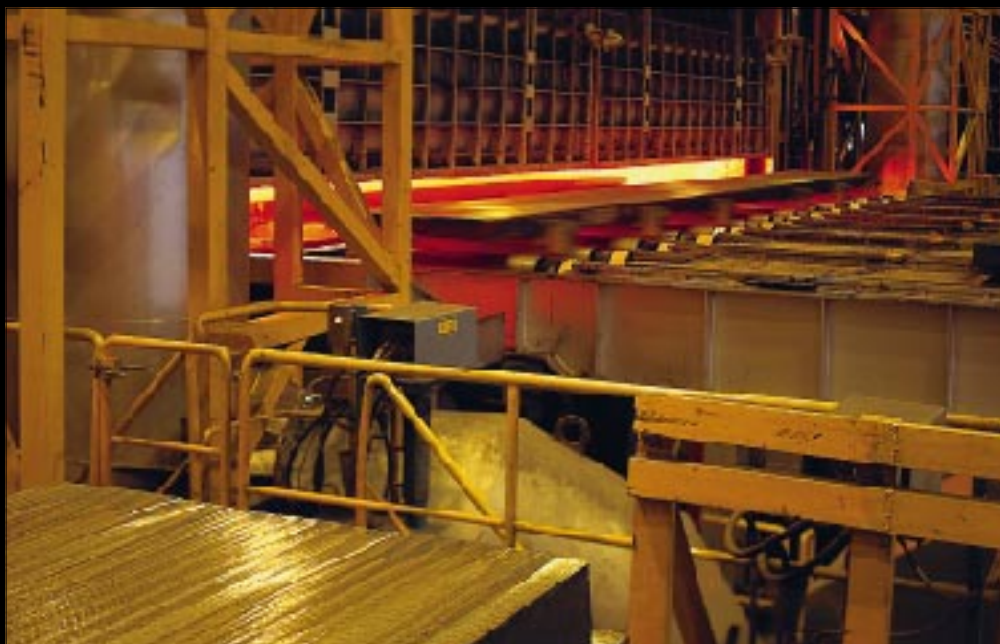
The temperature of the stainless steel slabs from the steel melting shop is raised in a walking beam furnace at the hot rolling mill. The furnace capacity is 120 tonnes per hour.
