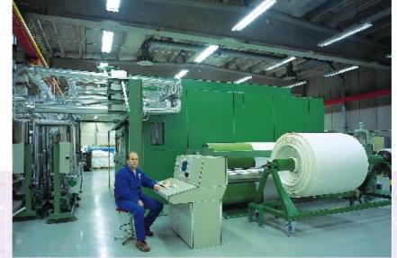
The finishing capacity of filter fabrics has been increased with an efficient new continuous heat-setting unit.
