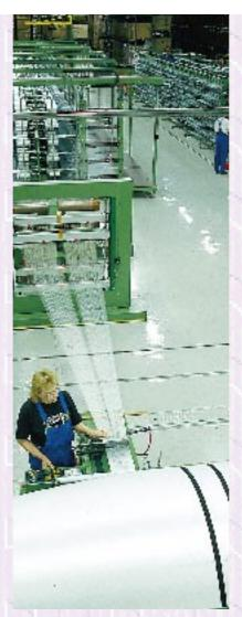
The new conical warping machine in the filter fabrics profit center serves the whole plant.
