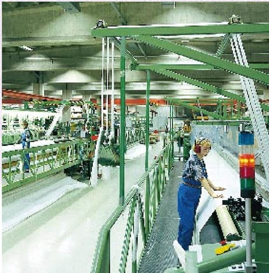
*The new efficient looms also provide additional capacity for press felt weaving, which is a bottleneck area.*
