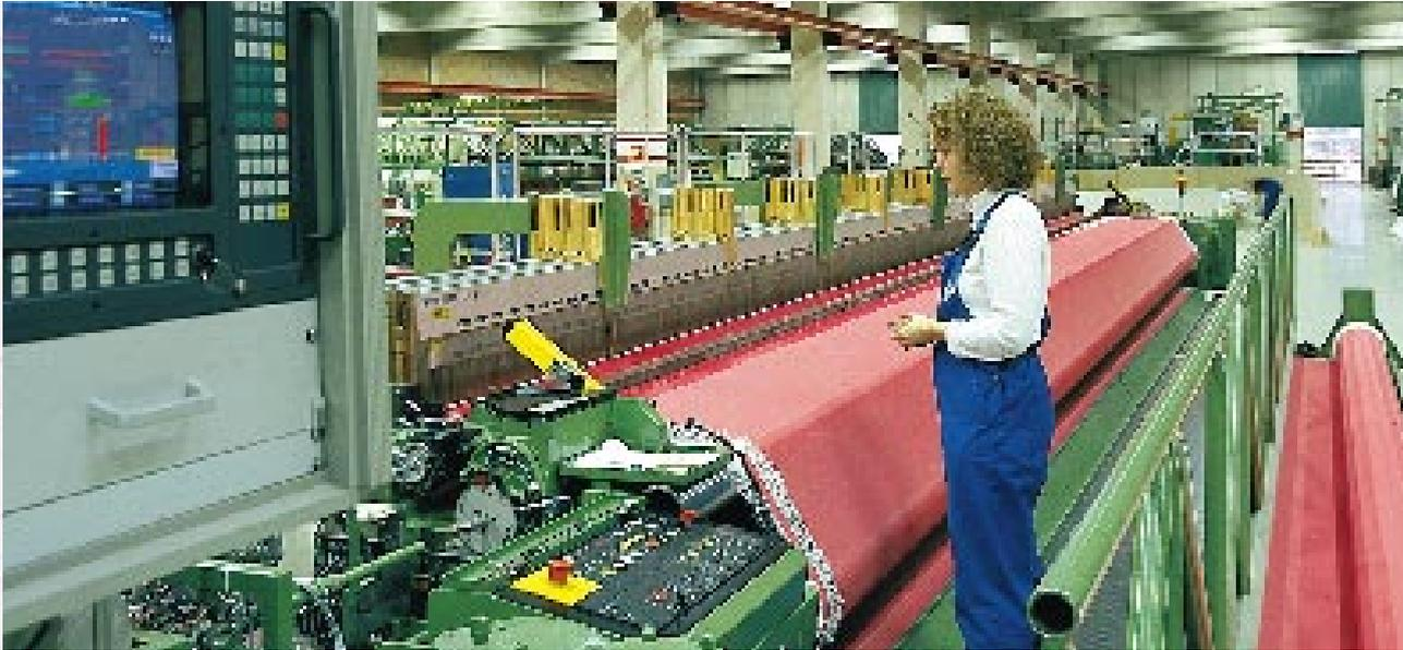
Capacity has been increased in the weaving mill of the Tampere plant. In the photo a new dryer fabric loom. Its speed is 75 strokes per minute, which is a lot more than that of the older machines.
