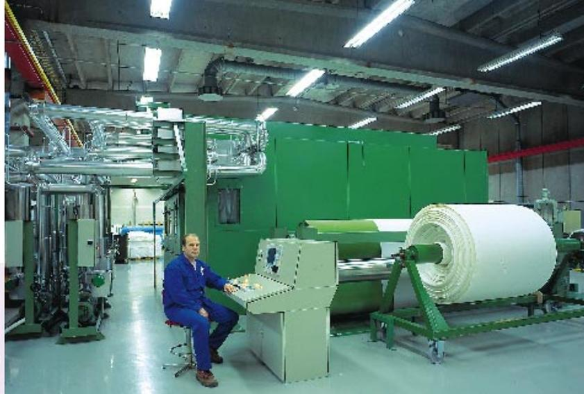
*The finishing capacity of filter fabrics has been increased with an efficient new continuous heat-setting unit.*
