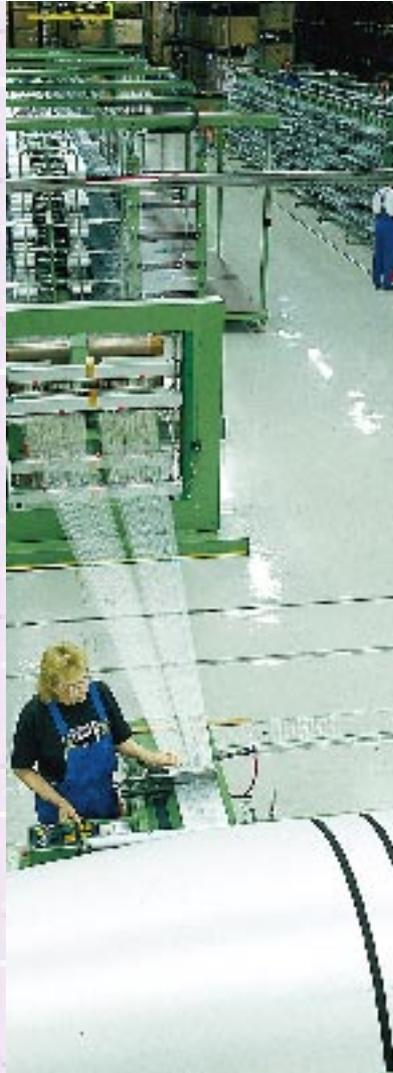
*The new conical warping machine in the filter fabrics profit center serves the whole plant.*
