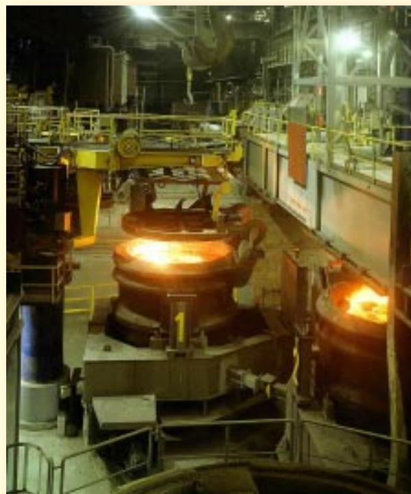
The new ladle metallurgy plant at the Raahe Steel Works opens the way to developing new steel grades.
