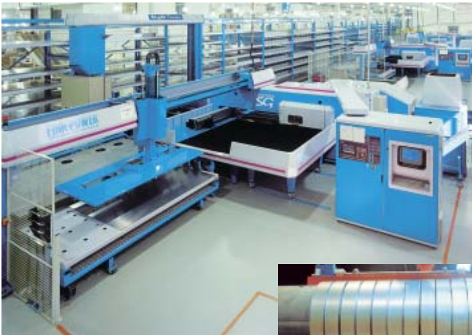
Finn-Power's Night Train flexible sheet metal manufacturing system, for which Asva supplies installation-ready machine parts.
