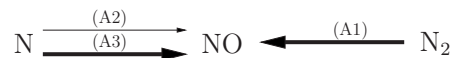
FIG. 23. Reaction flux diagram for Zeldovich mechanism of a partially premixed methane/air flame (Sandia flame experiment) at \chi_{Z,st}=50 \text{ s}^{-1} .
