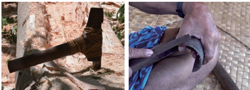
The to'i fafau, a hafted adze with a straight steel blade. The to'ū, a hafted adze with a curved steel blade.
