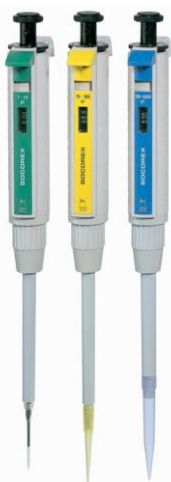
Fig.54 - Socorex® micropipettes in three different scales (1-10,10-100, 100-1000) [μl]
