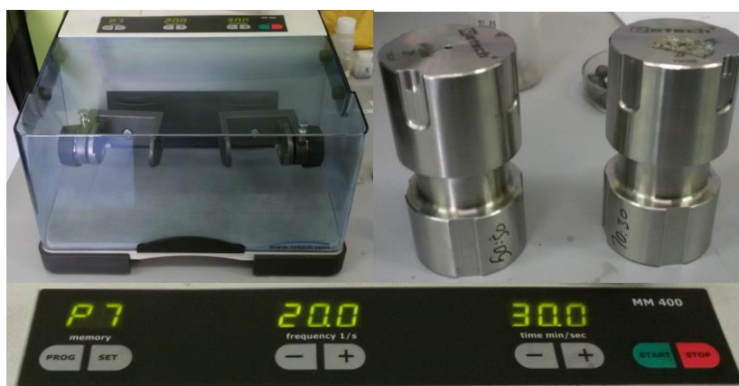
Fig.40 - In order from left to right: the 400 MM mixer mill, and the two milling cups. On the bottom a closer view of the user display
