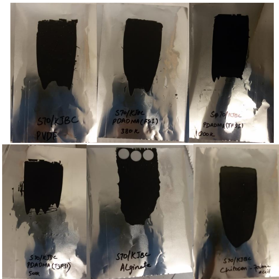
Fig.48 – The dry C/S/B preparation. In this example the case of the cathodes for long cycling with 10% of Binder.
