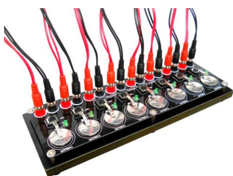
Fig.56 – 8 Channel board for cell testing [70]
