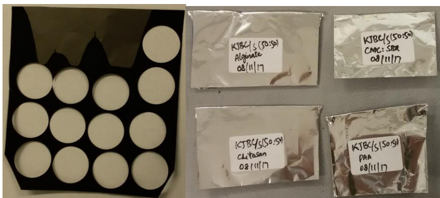
Fig.50 – On left An example of a good spreading of cathode ink, with 13 cathodes cutted (50:50 KJBC/S-PVdF). On the right the Al-bags that hosts the cathodes.
