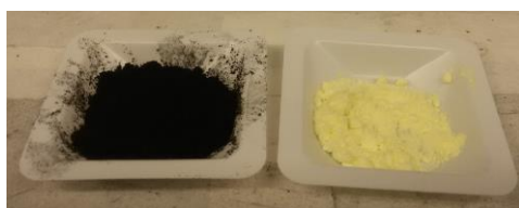
Fig.34 – As received raw materials Aldrich 99% sulfur and Akzo Nobel Ketjenblack EC-300 J carbon
