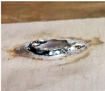
Spot weld on bottom plate
