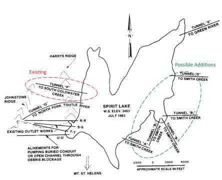
**FIGURE 5.2** Original suggested tunnel alignments. Existing tunnel alignment (circled in red) drains Spirit Lake to the west, through Harry's Ridge toward South Coldwater Creek. Possible tunnels might drain to the east, toward Smith Creek. SOURCE: Modified from USACE, 1983.
