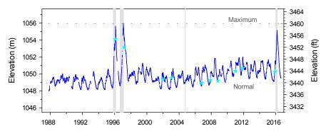
**FIGURE 5.7** Daily water-surface elevation of Spirit Lake from October 1987 through September 2016 from the U.S. Geological Survey gauge at Tunnel at Spirit Lake, Washington (14240304), with normal operating level and maximum elevation for safe operation. Gray vertical bars indicate periods of extended tunnel closure, and stars indicate the timing of the 10 largest 1-day inflows during the period of record. SOURCE: Grant et al., 2016b.
