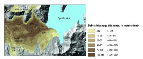
**FIGURE 2.5** Debris blockage thickness shown on topographic model derived from 2009 LIDAR survey. The debris thickness contours run along the old North Fork Toutle River in the northeast-southwest direction. SOURCES: Map derived by Adam Mosbrucker, USGS. Original data from Glicken et al., 1989.
