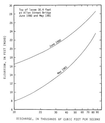
**FIGURE 4.2** Elevation-discharge curve for the Cowlitz River and Kelso-Longview, Washington. The June 1980 curve represents the post-eruption but pre-dredging condition of the river. By May 1981, dredging had lowered the bed of the river and correspondingly the elevation of the river surface. SOURCE: Lombard, 1986.
