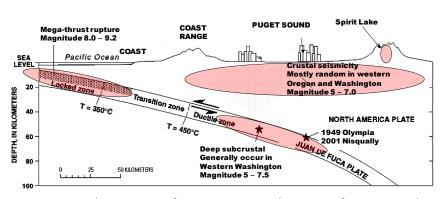
**FIGURE 4.3** Schematic map of seismic sources in the vicinity of Mount St. Helens. SOURCE: USACE, 2016b.
