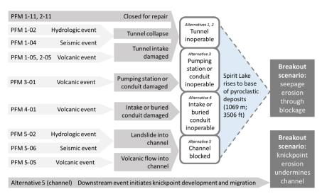
**FIGURE 5.1** Schematic depiction of potential failure modes, outcome of failure mode on infrastructure, and ultimate potential consequence of outlet system failure. SOURCE: Grant et al., 2016a.
