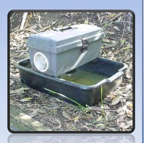
Gravid females of some species of mosquitos, such as Culex can be attracted to traps containing mixtures of oviposition stimulants like the extracts of rotten hay or grass. Female mosquitoes enter the trap and are forces into collection containers by a updraft fan.
