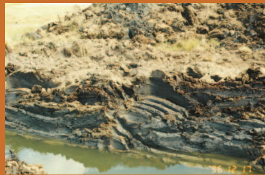
Potential acid sulfate soils (also called 'marine mud' or 'mangrove mud') are typically dark grey, wet and sticky. They can range from sand to clays. Photo: Queensland Acid Sulfate Soils Investigation Team (QASSIT), DERM
