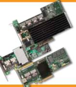
The MegaRAID SATA+SAS value line offers a mix of value and performance for internal SATA and SAS systems. These products feature 3Gb/s or 6Gb/s transfer rates, internal connectivity and support for both SATA and SAS drives.
