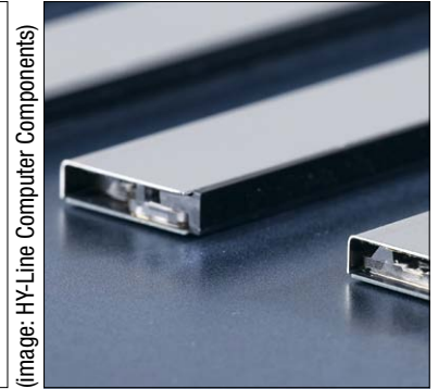
Figure 6. Sensor module from manufacturer Neonode, right opening for transmitter and receiver. (photo: Neonode)
