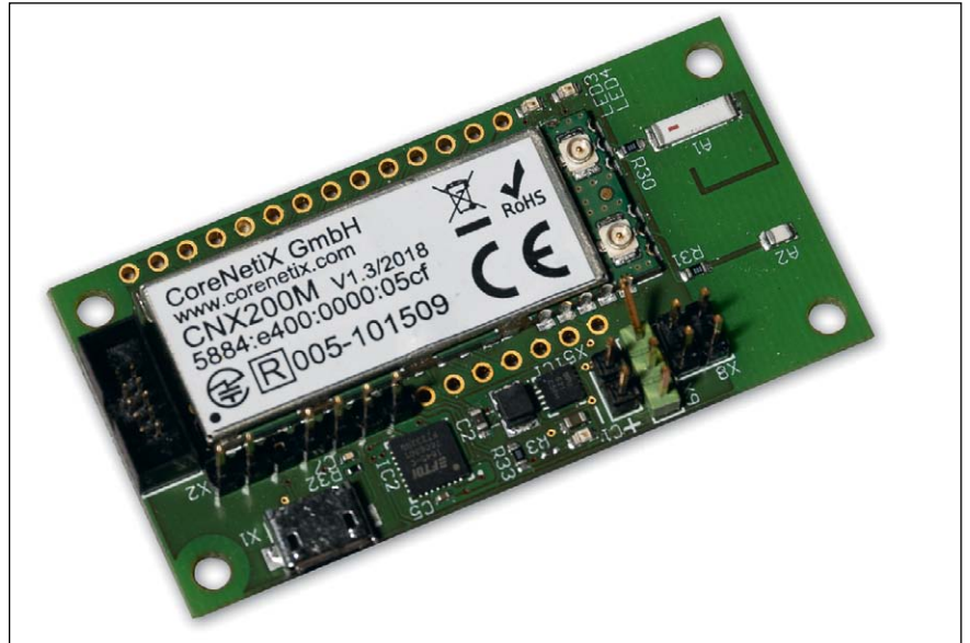
Figure 2. The IP500 wireless module CNX200 contains a microcontroller for the IP500 network stack and also the antenna. It fulfills all requirements for worldwide certification – for Europe (RED), India, Japan, USA (FCC), etc. (photo: IP500 Alliance)
