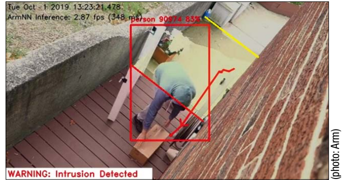
Figure 3: Inferencing in security cameras will enable faster actions, by detecting the presence of an unknown person, identifying a package and inferring whether the person is delivering the package or potentially stealing it.
