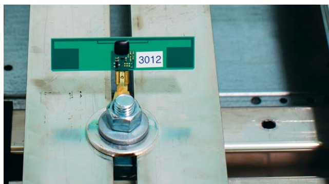
Figure 1. Passive RFID temperature sensor on a screwed join in switchgear. (photo: Fraunhofer IPMS)
