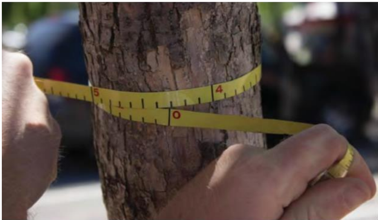
Record the d-tape reading where the 0 mark overlaps (reading is 4.3)
