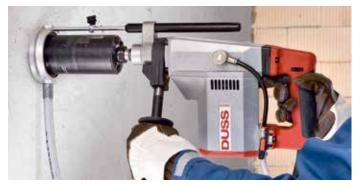
Wet socket sinking in concrete with water extraction
