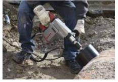
Dry drilling in a plastic pipe, hand-held
