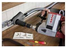
Clean wet drilling in concrete with DUSS suction cup, hand-held
