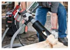
Drilling in wood with dust extraction, hand-held
