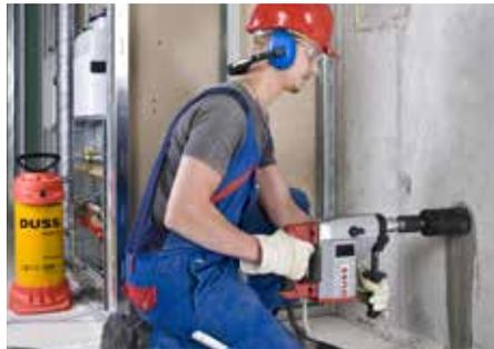
Electrical socket sinking in concrete – wet, hand-held
