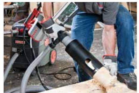
Drilling in wood with dust extraction, hand-held
