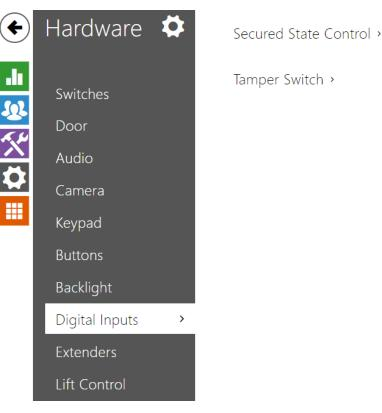
In this configuration section set the parameters associated with digital inputs and their interconnections with other intercom functions.
