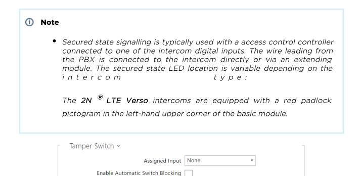
The tamper switch equipped models help detect opening of the device cover and signal this event as **TamperSwitchActivated**. The events are written into a log and read out via HTTP API (refer to the **HTTP API** manual).
