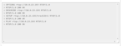
The External IP Camera Log displays the RTSP communication with the selected external IP camera including failures and error states if any.
