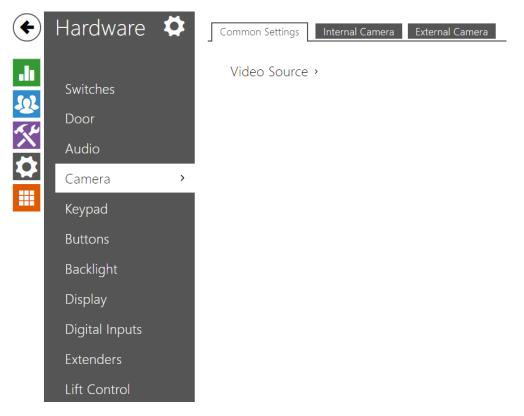
This menu is only available in the **2N LTE intercom** models that are equipped with an internal camera or can be connected to an external camera. The camera signal can be streamed directly into the call via a videophone, sent by E-mail, streamed via ONVIF /RTSP to another device (a video surveillance device, e.g.), or simply HTTP downloaded from the intercom in the JPEG format.
