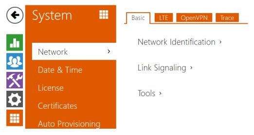
The **2N LTE intercom** gets connected to the LTE network via a SIM card. The access data (APN, access name and password) are configured automatically. To change the LTE access data configuration, use SMS (refer to the Installation manual) or the LTE tab of the web configuration interface (see below).
