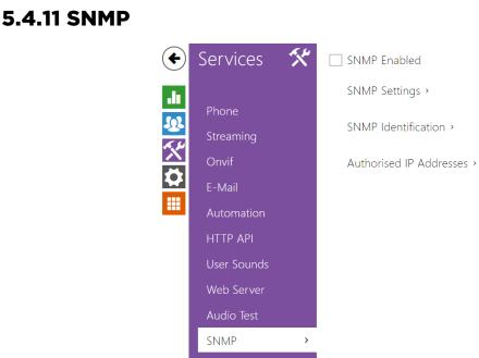
The **2N LTE intercoms** integrate a remote intercom supervision functionality via the SNMP. The integrated SNMP agent becomes available when the **Enhanced Integration** licence key is added. The intercoms support the SNMP version 2c.
