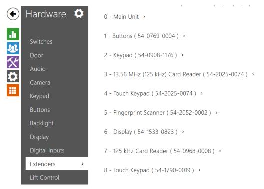
The **2N<sup>®</sup> LTE Verso** intercoms can be enhanced with extending modules connected to the intercom basic unit. The following modules are available:
