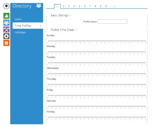
Such intercom functions as outgoing calls and RFID card/numeric code access, for example, can be time-limited by being assigned a **time profile**. By assigning a time profile you can:
