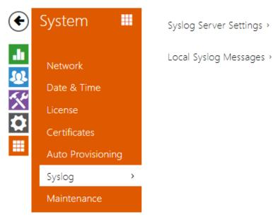
The **2N LTE intercoms** allow you to send system messages to the Syslog server including relevant information on the device states and processes for recording, analysis and audit. It is unnecessary to configure this service for common intercom operation.
