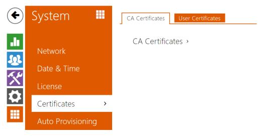
Some **2N LTE intercom** network services use the Transaction Layer Security (TLS) protocol for communication with other LAN devices to prevent third parties from monitoring and/or modifying the communication contents. Unilateral or bilateral authentication based on certificates and private keys is needed for establishing connections via TLS.
