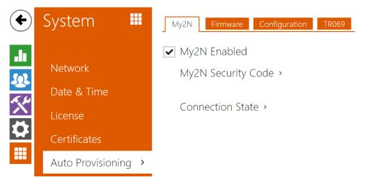
The **2N LTE intercoms** help you update firmware and configuration manually, or automatically from a storage on a TFTP/HTTP server selected by you according to predefined rules.
