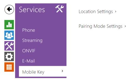
The 2N LTE intercoms equipped with the Bluetooth module allow for user authentication via the  $2N^{\textcircled{R}}$  Mobile Key application available to devices with iOS 12 and higher (iPhone 4s and higher phones) or Android 6.0 Marshmallow and higher (Bluetooth 4.0 Smart supporting phones).
