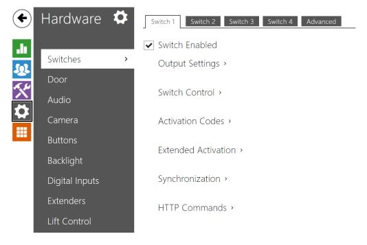
Switches provide a very flexible and efficient control of such intercom peripherals as electric door locks, lighting, additional ringing signalling, and so on. **2N LTE intercoms** allows you to configure up to 4 (depending on model types) independent all-purpose switches.
