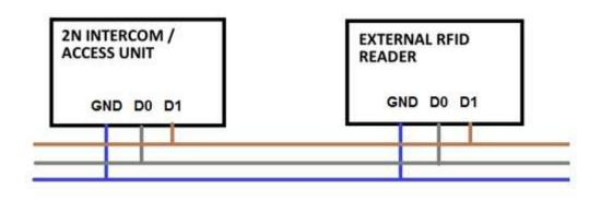
Recommended Wiring Diagram for Reader with Bus Driver
