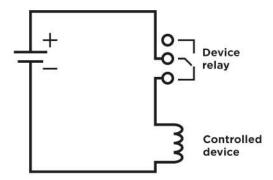
Wiring diagram for the controlled device's electric circuit opening
