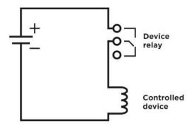
Wiring diagram for the controlled device's electric circuit closing
