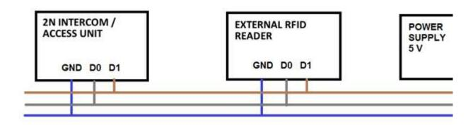
Recommended Wiring Diagram for Reader with Open Collector (OC) Output
