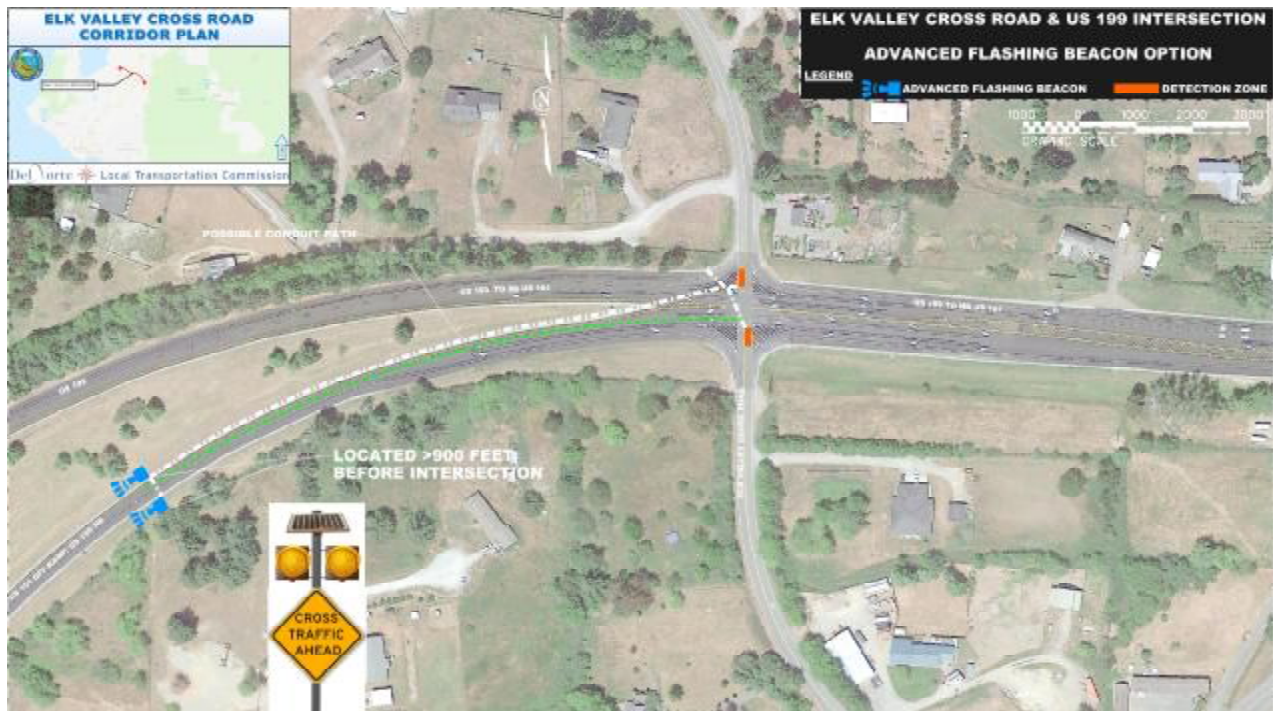
Figure 6: Advanced Flashing Beacon Conceptual Layout
