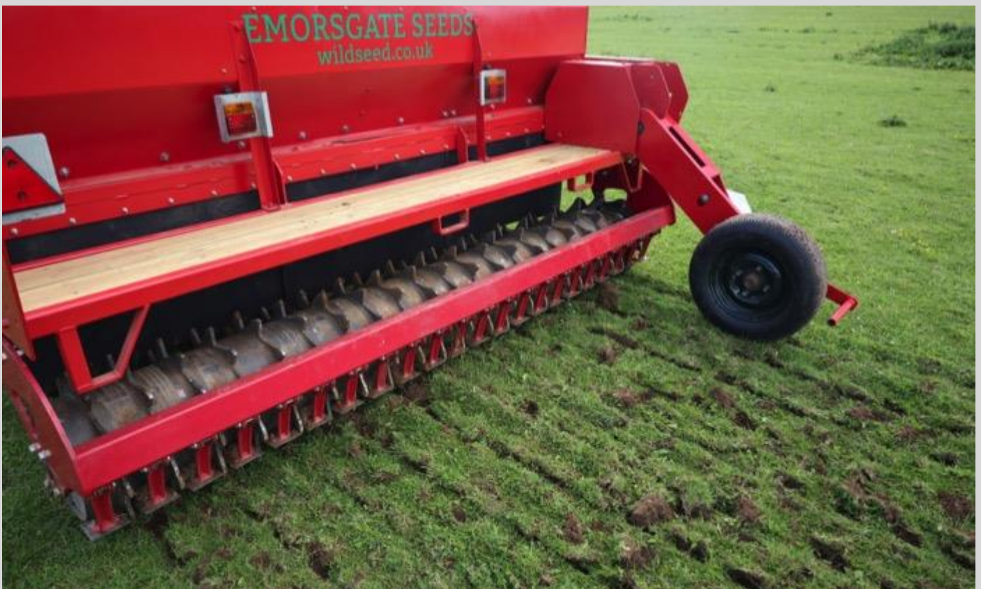
MEADOW RESTORATION: 3m roller feed seed box mounted on 3m discs surface sowing a meadow mixture at 2g/m 2 onto the surface of scarified species poor grassland
