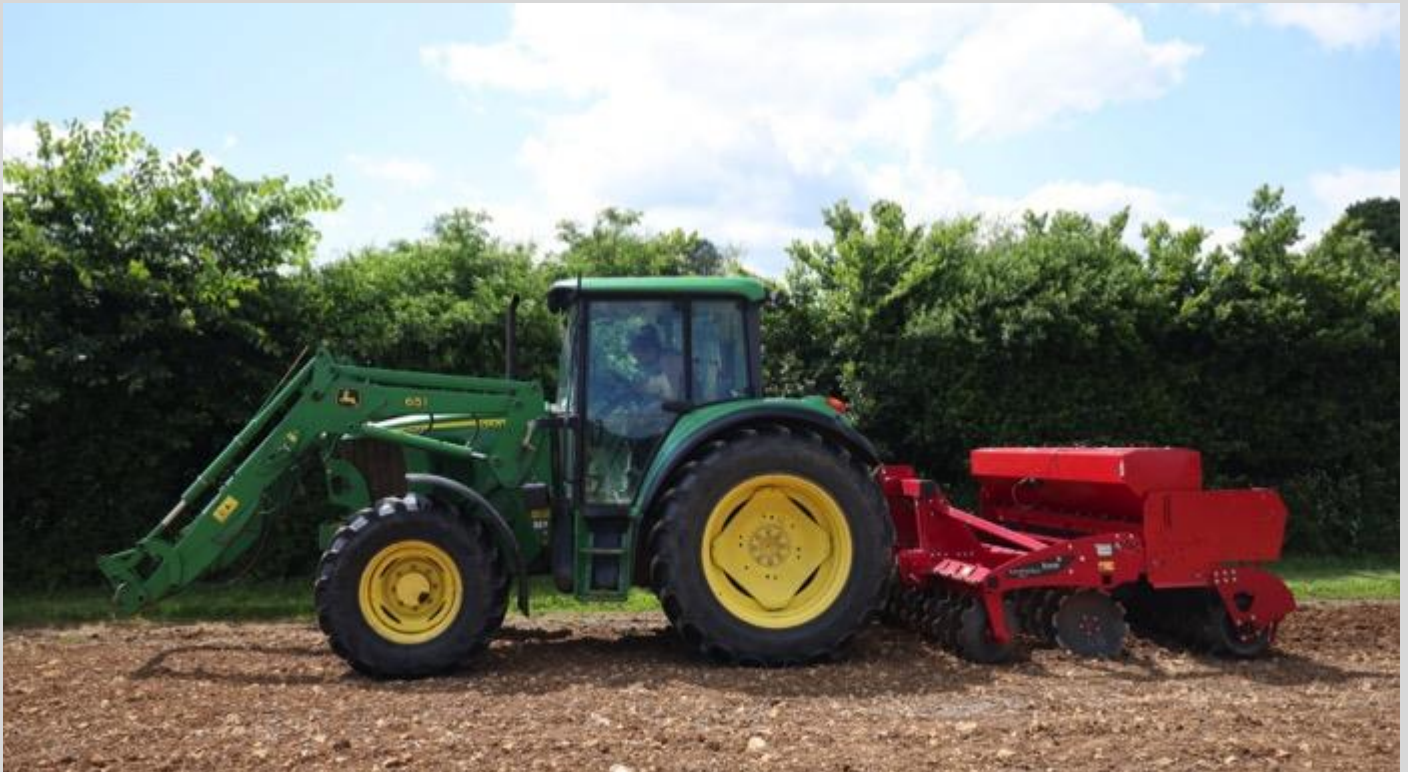
MEADOW CREATION: 3m roller feed seed box mounted on 3m discs surface sowing a meadow mixture at 2g/m 2 onto the surface of prepared bare soil
