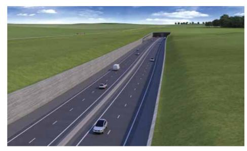
Figure 5.22: Approach option with vertical retaining walls
