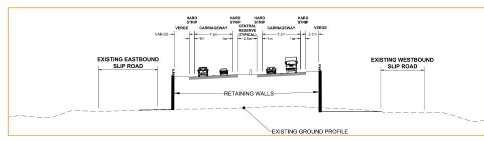
Figure 5.46: The cross-section above illustrates how the flyover would be constructed between the existing approaches to Countess roundabout which would then become the slip road connections between the new A303 and the A345.
