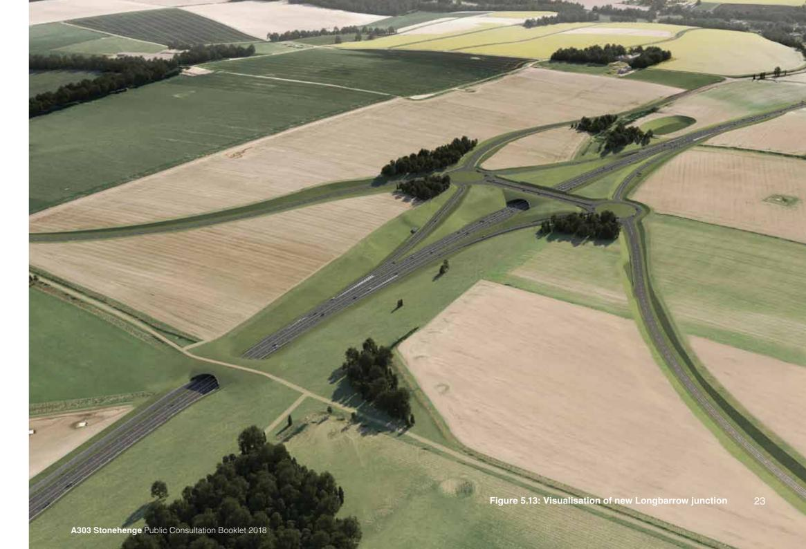
The new Longbarrow junction would comprise slip road connections into two roundabouts linked by a green bridge (No. 3) over the new A303. While serving to carry A360 traffic, the bridge would also be designed to soften its appearance within the landscape.
