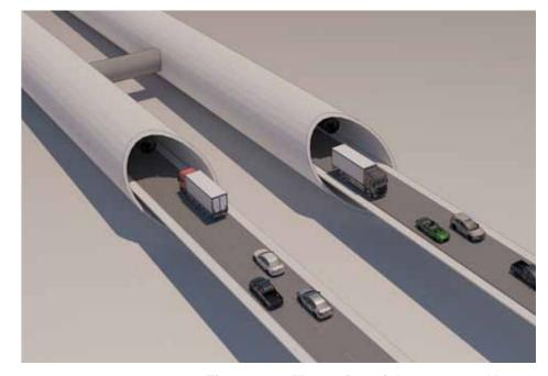
Figure 5.37: Illustration of the two tunnel bores
