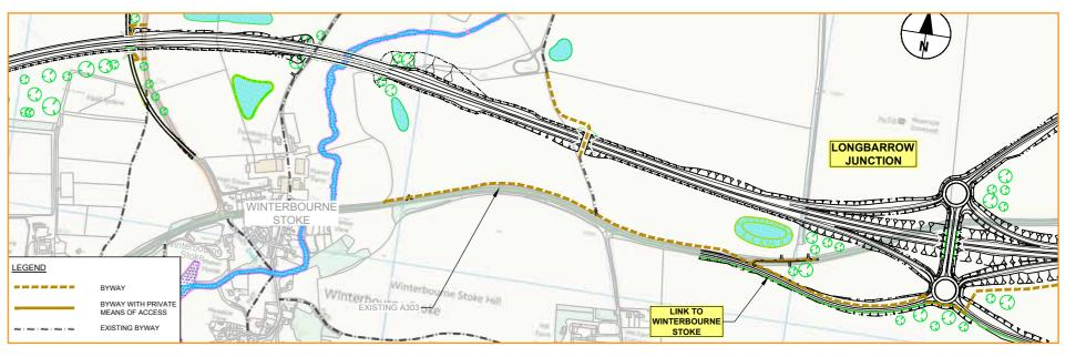
Figure 5.15: Link road from new Longbarrow junction to Winterbourne Stoke
