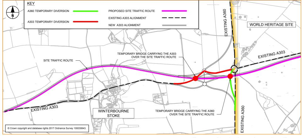
Figure 6.12: Plan showing continuous site traffic route
