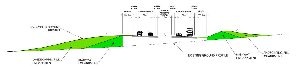
Figure 5.5: Typical cross section
