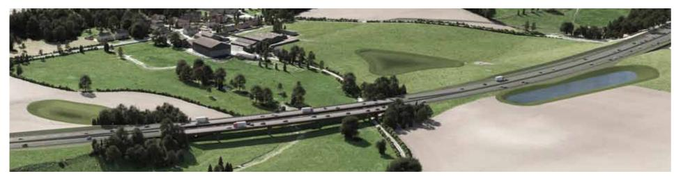
Figure 5.12: Road drainage infiltration areas either side of the River Till
