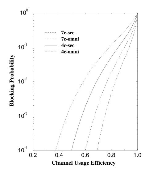
Channel usage efficiency  $\eta_C = \rho(1 - B(\rho, m)/m)$  for different trunkpool schemes; 416 channels.
