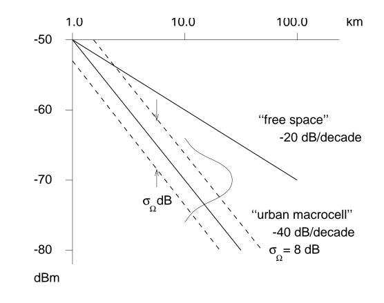
Path loss and shadowing in a typical cellular environment.
