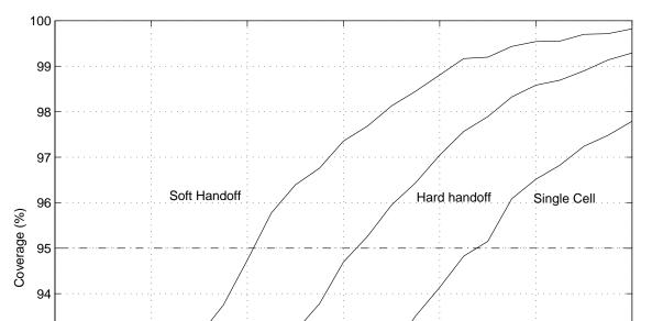
Typical handoff<sub>3</sub>gain for hard and soft handoffs. In this plot shadow margin is defined as  $M_{shad} + G_{HO}$ , where  $M_{shad}$  is the shadow margin required for a single cell. We also plot the area averaged outage as opposed to the edge outage.
