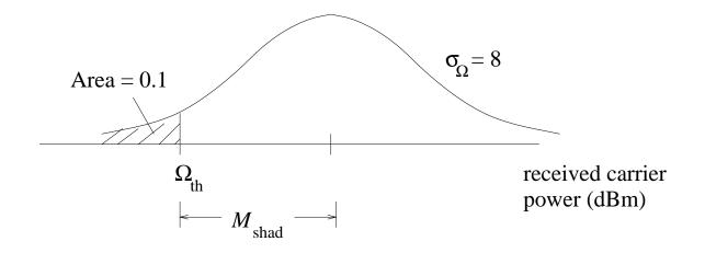
Determining the required shadow margin to give  $P_E = 0.1$ .
