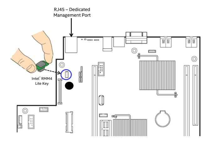
Figure 59. Intel® RMM4 Lite Activation Key Installation
