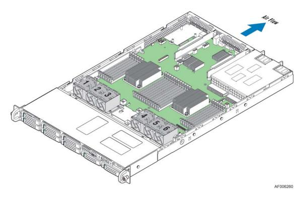
Figure 25. System Air Flow and Fan Identification
