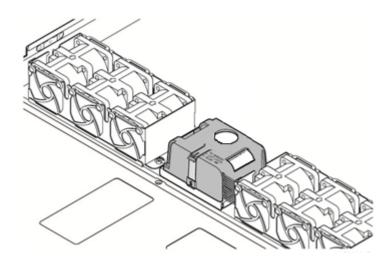
Figure 52. Support for dual Intel<sup>®</sup> RAID Maintenance Free Backup Units (Optional Accessory)
