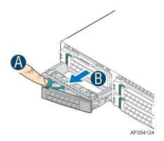
**Note:** To ensure proper system air flow requirements, all front drive bays must be populated with a drive tray. Drive trays must be installed with either a drive or supplied drive blank.
