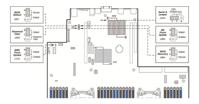
Figure 6. System Reset and Configuration Jumpers
