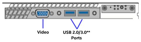
Figure 53. Front I/O Panel Features
