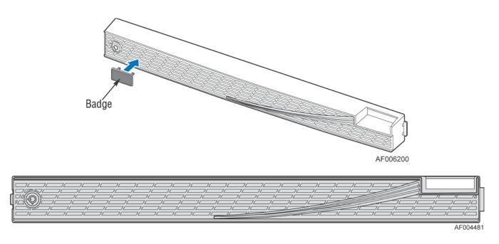
Figure 12. Front Bezel accessory with optionally installed wave feature
