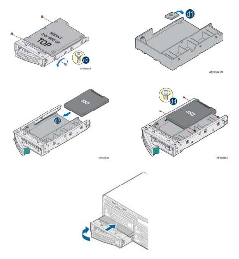
Figure 31. 2.5" SSD mounted to 3.5" Drive Tray
