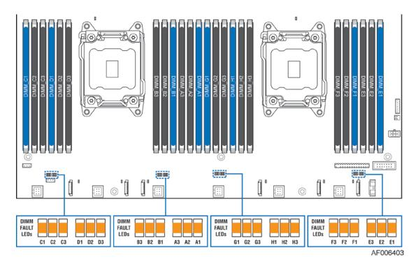
Figure 5. DIMM Fault LEDs
