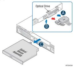
Figure 35. Optical Drive Installation
