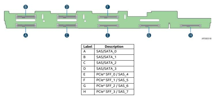
Figure 43. 8 x 2.5" Drive Combo SAS / PCIe\* SFF Backplane - front view
