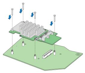
connector (labeled "SAS Module") on the server board.
