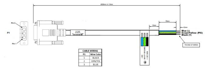
Figure 24. DC Power Cord Specification
