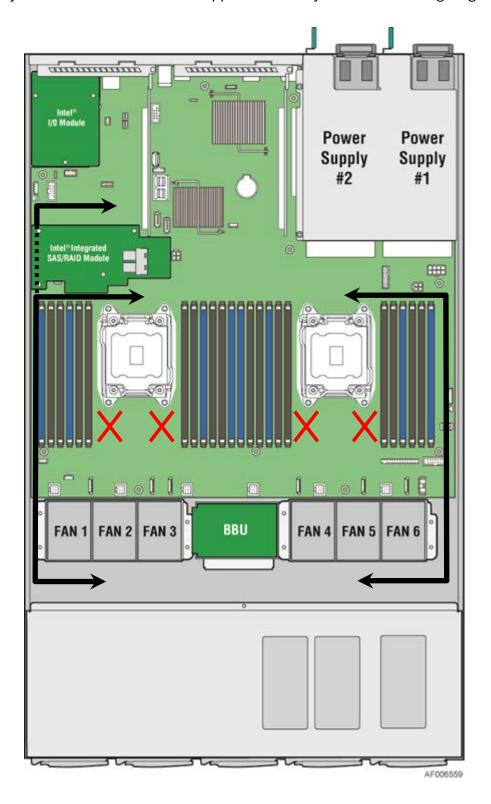
Figure 19. System Cable Routing Channels
