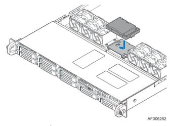
Figure 51. Support for single Intel® RAID Maintenance Free Backup Unit (Standard Option)
