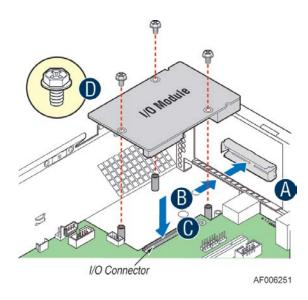
Figure 58. Intel® I/O Module Placement
