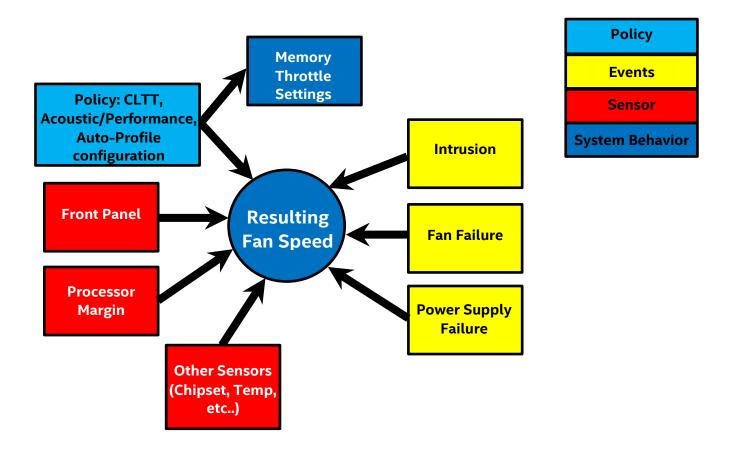
Figure 26. Fan Control Model
