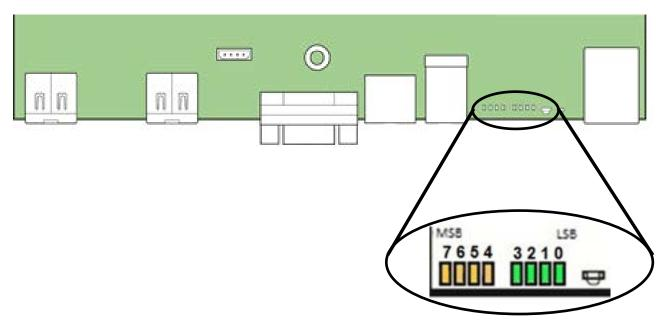
Figure 60. POST Diagnostic LED Location
