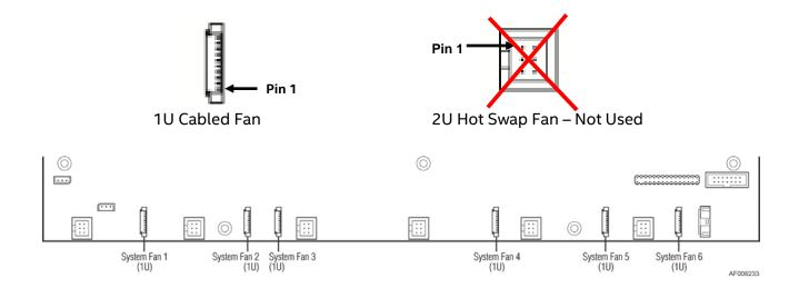
Figure 28. System Fan Connector Locations on Server Board
