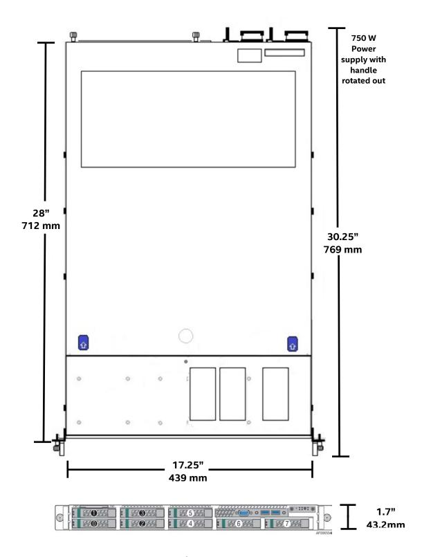
Figure 16. Chassis Dimensions
