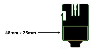
Figure 18. Pull-out Tab Label Emboss Dimensions
