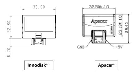
Each installed SATA DOM plugs directly into one of the white single port SATA connectors on the server board, which provide both power and I/O signals.
