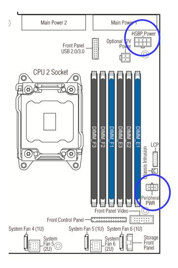
Figure 33. Server Board Peripheral Power Connectors
