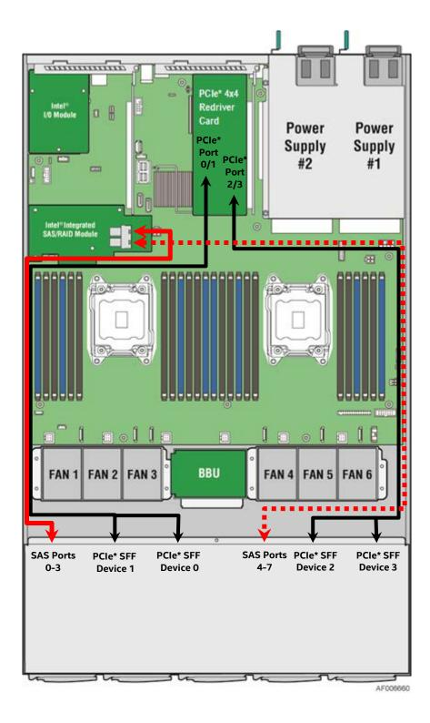
Figure 40. Combo Backplane Cable Routing - PCIe\* SFF + SAS
