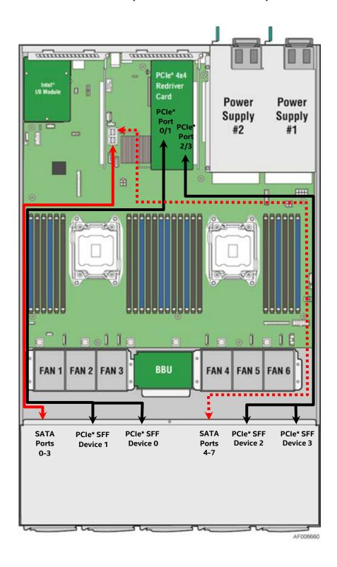
Figure 41. Combo Backplane Cable Routing - PCIe\* SFF + SATA
