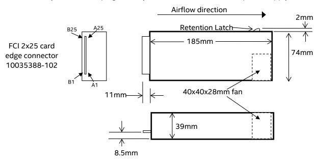
Figure 22. 750W AC Power Supply Module Mechanical Drawing
