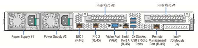
Figure 7. Back Panel Feature Identification
