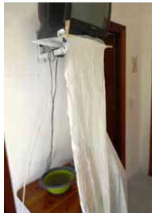
Figure 2. The tank and muslin containment system in construction. Clothes pegs were used to secure the muslin.
