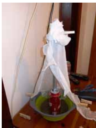
Figure 9. Emergence tank mark 2. Television abandoned and vertical support provided by a used beer can.
