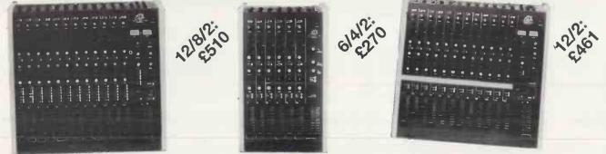
★ 6/4/2 ★ jack mic & line inputs ★  $4 \times$  send/return to record ★ Breakjacks ★ 3 band eq ★ Aux 1 switchable pre/post ★ Aux 2 s/r with full return routing ★ Monitor vol & pan on in-line channels ★ PPI ★ 2 track playback ★ 100mm faders ★ Separate Aux 1 and Mix phones outputs ★
