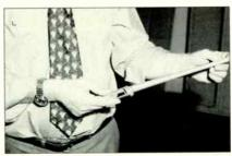
A Series V arm-tube ready to be tumbled in a bath of plastic chips to take off any rough edges.
