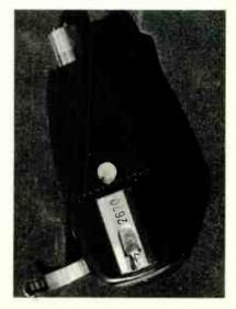
The bullion-plated SPU Gold weighs in at a massive 32gms and that's without the highgain step-up transformers of its predecessors.
