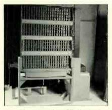
Alastair's modified Quad ESL 63s, showing the brass cross-braces used to stiffen the frames.
