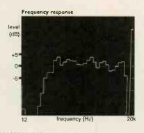
RDM1s have only a single peak instead. The overall impedance measured  $6.9\Omega$  and sensitivity was 87dB, not bad for a small stand mounter. About 60watts should suffice to drive the KEFs loud. **JM**
