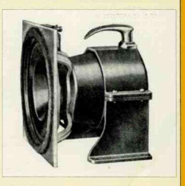
The permanent magnet PM4 drive unit shown here succeeded earlier Lowther mains energised designs. To achieve high flux density though, the rear magnet assembly had to be huge. It needed special support as a result. Lowther units had very high sensitivity and are still in demand today because of it.
