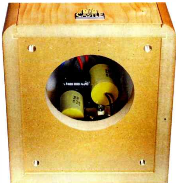
A large reflex port in the base of the cabinet exhausts onto a base plate. A small air gap between them provides resistive damping. Inside, Castle use high quality polypropylene capacitors in the crossover.
