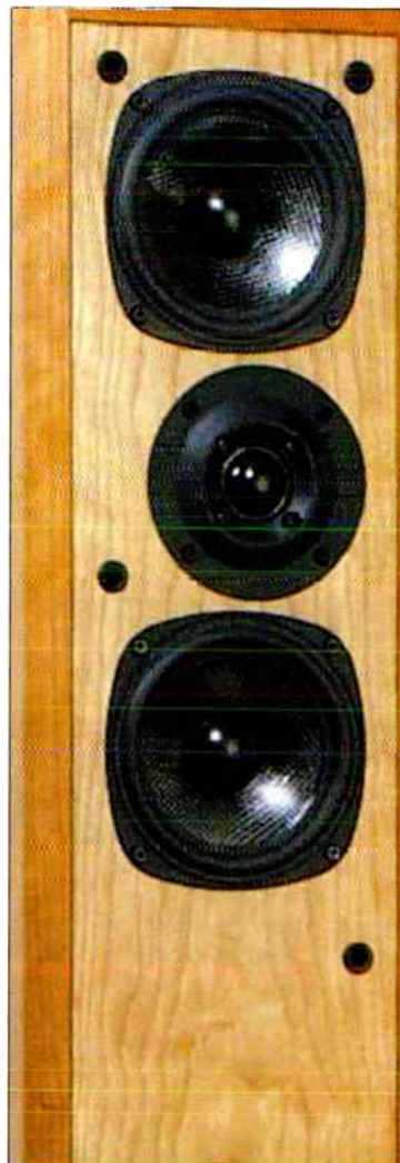
A fabric dome tweeter sits between two carbon-fibre bass/midrange units in d'Appolito arrangement. This improves vertical dispersion.
