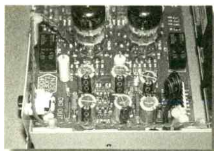
Valves in a modern Philips circuit board
