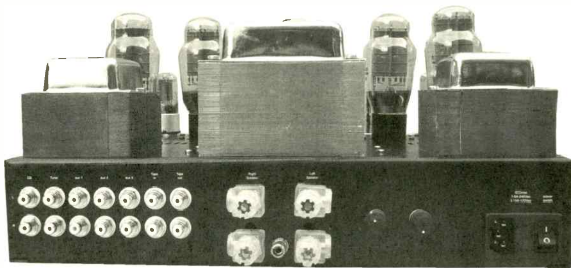
Rear view of the 2A3 PSE integrated amplifier showing heavy duty 'speaker terminals (centre), six inputs and tape out, plus mains switch (right).
