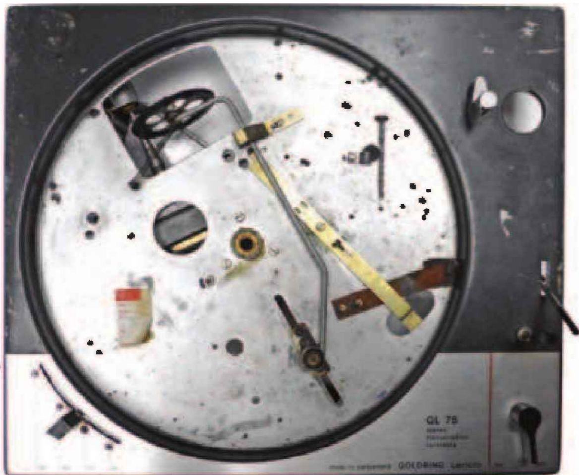
With the platter removed, the simplicity of the (G)L75 design becomes apparent. In addition to the bearing housing and speed control linkage you can see the platter 'brake' (roughly 'three o'clock' in the platter cavity).
