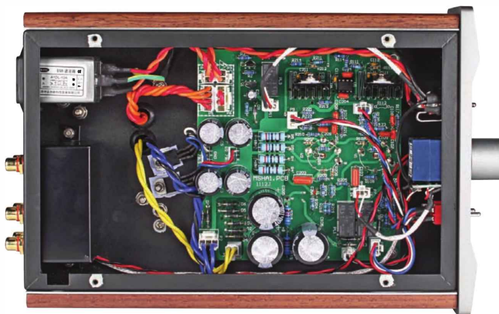
The Fosgate has neat and tidy internal wiring with the high-current video buffers clearly visible at the top of the circuit board.
