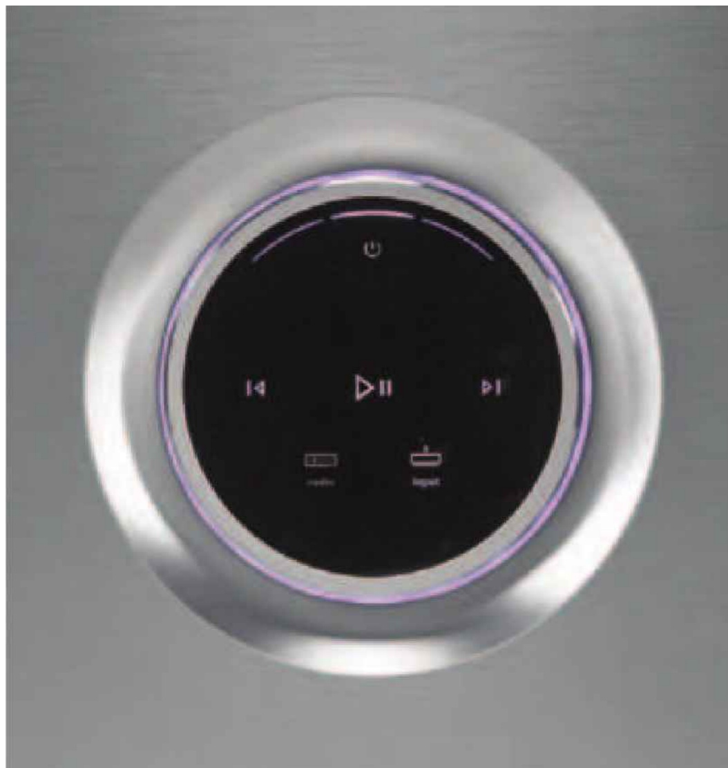
The top-mounted touch-sensitive dial controls volume, inputs and radio pre-sets.
