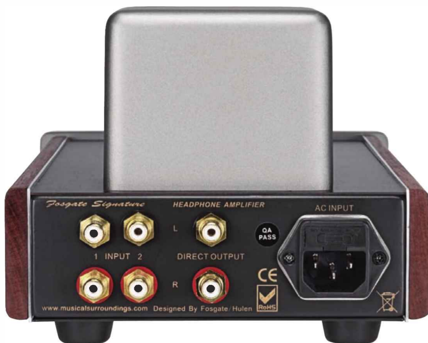
The rear panel includes two inputs on RCA jacks plus a direct output which by-passes the Fosgate's volume control for connection to a pre-amp or integrated amplifier.
