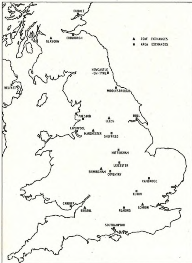
In addition to the 23 exchanges shown there will be 27 hypothetical exchanges, forming part of the six zone-centre exchanges FIG. 1—AUTOMATIC TELEX EXCHANGES IN THE INITIAL PROGRAM
