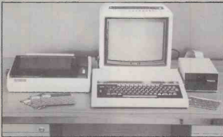
Apple IIe with Apple single disc drive and Epson RX-80 printer, driver a domestic TV display.
