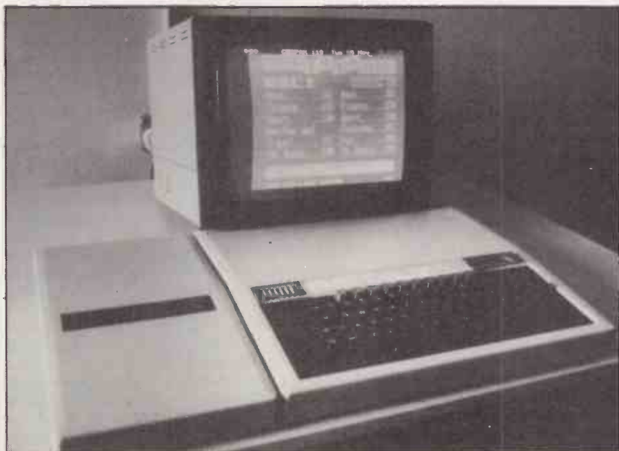
The BBC Micro and teletext adaptor, with the main Ceefax page on the screen.
