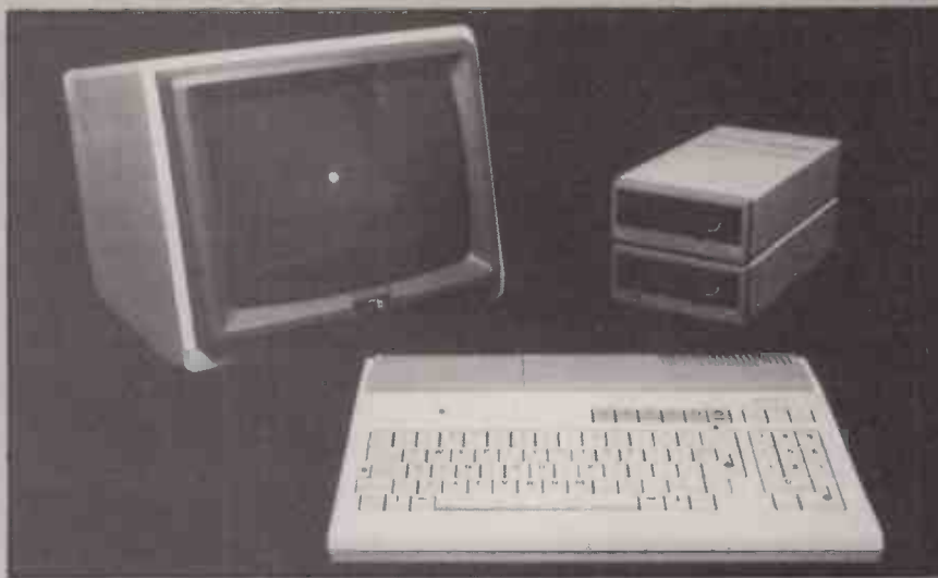
Alphatronic PC micro with 64K standard RAM, £339; disc drive with CP/M operating system, £380.
