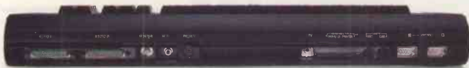
Input/Output Monitor, Hi-Fi, Power, TV, Centronics, Cassette Mic and Ear, and two Joystick ports all come as standard; the twin RS232 ports are available as expansions.
