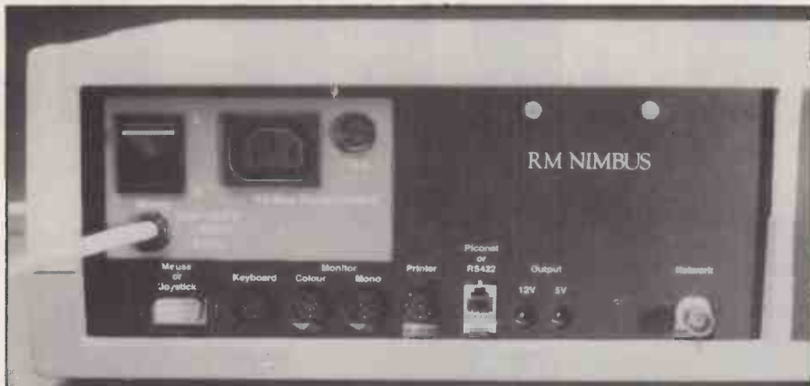
The I/O ports are situated at the back of the system box. The Piconet interface, sixth from the left, allows you to daisy-chain up to 30 peripherals to the Nimbus.
