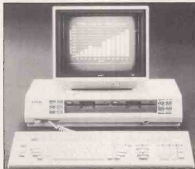
Epson's QX-16 is a dual 8088 and Z-80 processor machine running under MS-DOS and CP/M. There is also an optional IBMulator board. Standard features include 156K RAM expandable to 512K, and dual 5.25in. floppies offering 360K or 720K per disc. The cost has yet to be announced. More on 01-902 8892.
